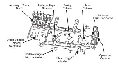
1) Auxiliary Contact Block: Auxiliary Contact Block contains the changeover switch contacts in combination of 4 units of 1NO+1NC each. Auxiliary contact block reflects the breaker ON/OFF state in control circuit.
