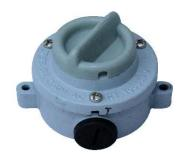
KAYCEE Rotary Toggle Switches type RT-1000D incorporates a switch protected in a metallic housing, suitable for outdoor installation as they are weather tight. These switches are recommended for their quick installation and use in all weather conditions. Installation is by fixing two suitable screws. Easy wiring is through a conduit entry size 20mm.
