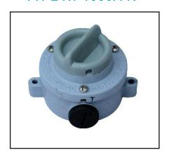
KAYCEE Rotary Toggle Switches type RT-1000A-N incorporates a switch protected in a metallic housing, suitable for outdoor installation as they are weather tight. These switches are recommended for their quick installation and use in all weather conditions. Installation is by fixing two suitable screws. Easy wiring is through a conduit entry size 20mm.
